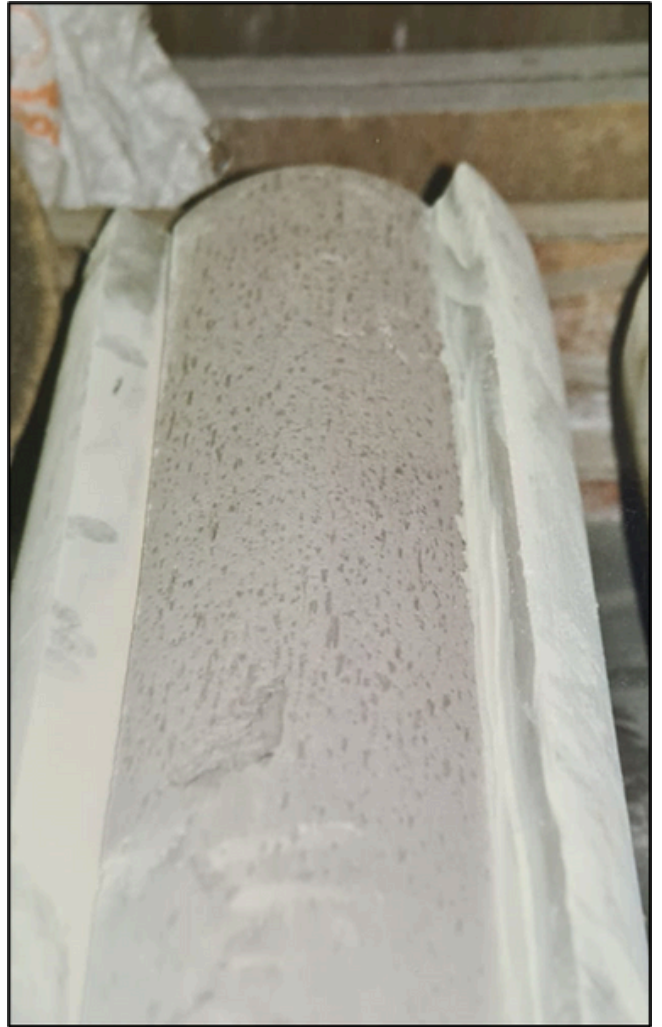
Modified SDP for pumping with thixotropic properties to facilitate installation
