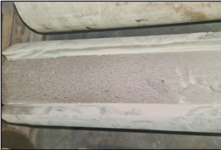
Modified SDP for pumping with thixotropic properties to facilitate installation
