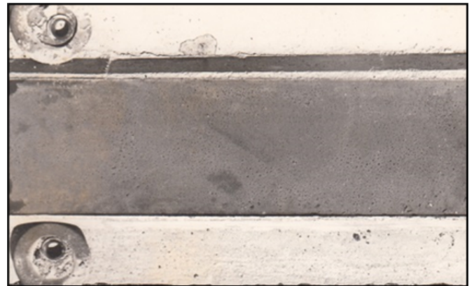
SDP Grout with full effective bearing area
