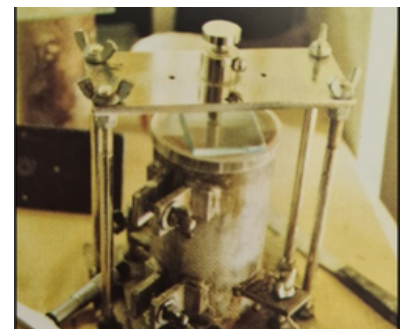
Dimensional stability test US Corp of Engineers GPR 6621-82A
