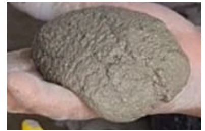
Thixotropic Grout is stagnant without energy
